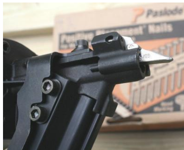
Probing tip makes it easy to find the holes in the metal connectors
