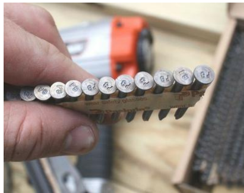
Code approved hardened nails with head markings
